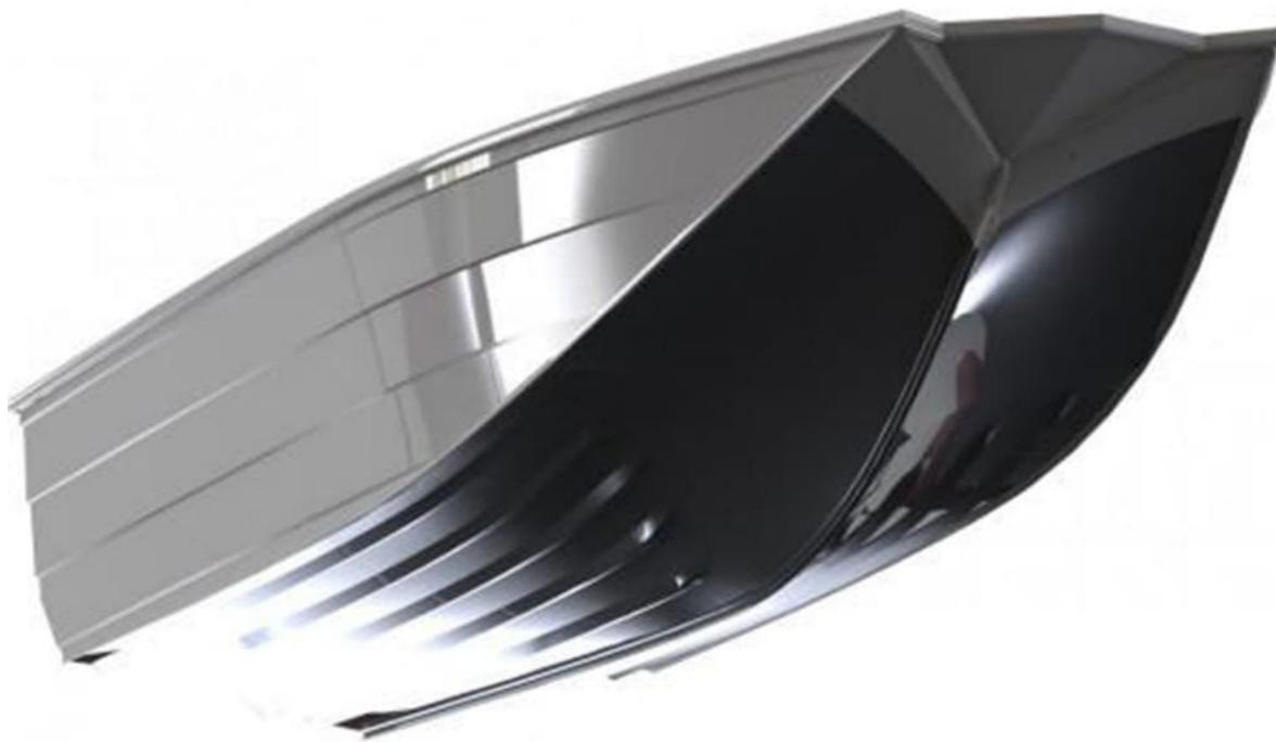
The hull, introduced in 2017, brings big benefits above the waterline. Its forked bow – which carries the wide beam all the way forward – creates significantly more internal space enabling Quintrex to include a larger seating area in the Freestyler bowriders, and a bigger casting deck in Quintrex Frontier fishing rigs.
