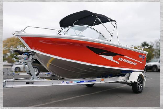
The Quintrex Fishabout Pro range also has added more cockpit space by removing the outboard engine well and replacing it with a transom-mounted pod, with duckboards to either side.
