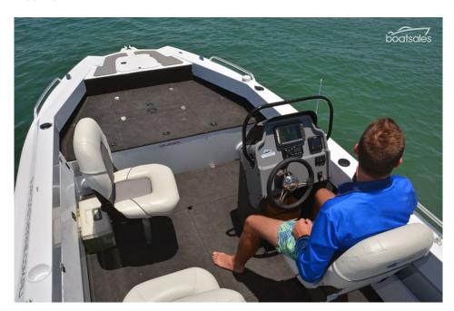
The casting platform aft of the anchor well is situated 400mm above the rear cockpit floor. Beneath it is a series of storage lockers for safety gear, and a platform in the forepeak locker for an electric trolling motor battery.
