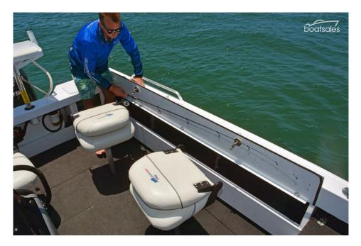
In our test boat this good-sized cockpit was flanked by a side storage pocket on the port side and the optional full-length rod locker over to starboard, beneath the 112mm wide side coamings.
