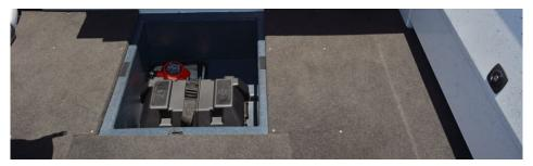
Beyond that, there is another underfloor storage locker which houses the battery with a bilge pump alongside it. The battery is secure in this location, but we would still prefer it to be situated on a shelf above the floor level, clear of any water that may flood the cockpit.
