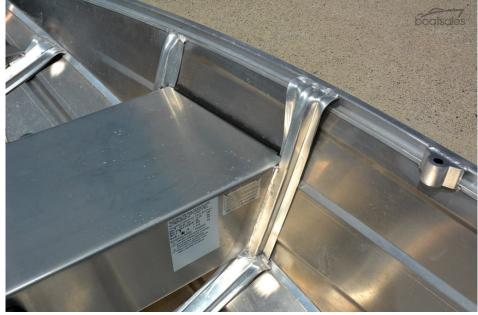
The thwarts are also wider and deeper than you will find in most cartoppers, and filled with enough foam for the hulls to achieve a Basic Flotation standard.
