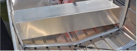
Standard features within the boat itself includes bow and stern carry handles, a double towing eye for attaching a safety chain in addition to the winch strap/cable, welded, reinforced rowlock blocks, a V-shaped internal transom structure with diagonal support brace, the aforementioned oversized bench seat-thwarts (380mm wide), and a total of seven internal crossribs, four of which rise up to the gunwale from the internal chines.
