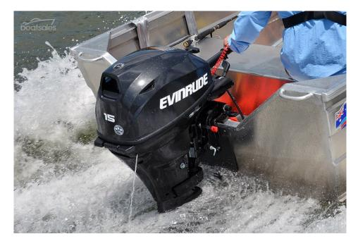
The tiller-operated, twist-grip throttle Evinrude 15hp was easy to use and delivered strong, consistent power from idle through to a wide-open throttle top speed of 21.1 knots — which is ample for applications ranging from tender through to backwater car-topper fishing rig.
