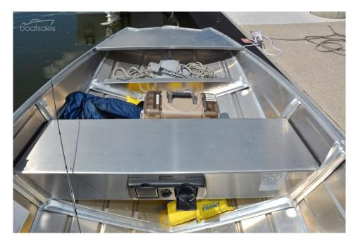
Built into the forward seat thwart you'll find a handy glove-box for stowing the car keys, cell phones, etc. The box also incorporates two flip-out drink holders.
