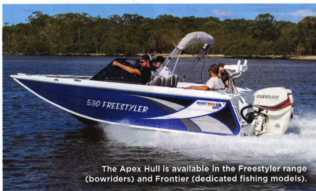
The new Apex Hull is carried further aft to maintain contact with the water when on the plane, which creates a smoother ride.
