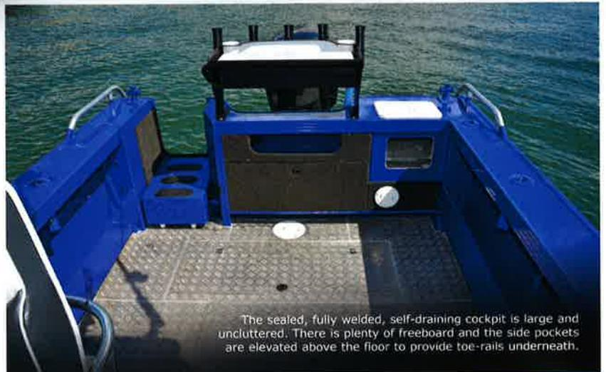
The sealed, fully welded, self-draining cockpit is large and uncluttered. There is plenty of freeboard and the side pockets are elevated above the floor to provide toe-rails underneath.
