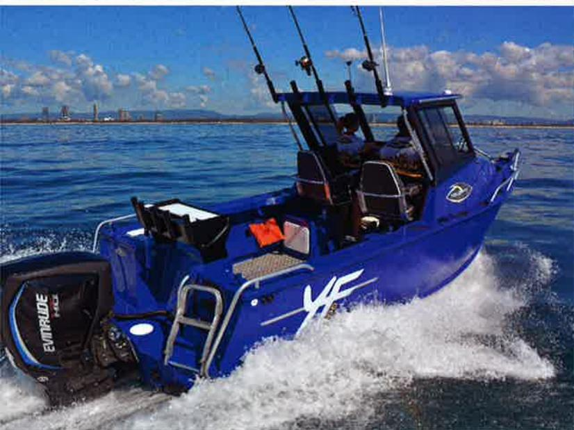
**Top:** The transom layout works very well. The batteries are sheltered in a locker behind the transom wall, while overhead is an open shelf for stowing lures. Note how the starboard-side transom door has been laid flat to create a useful step. The port-side livebait tank has a capacity of 60 litres and a front viewing panel so you can easily check the condition of your baits.
