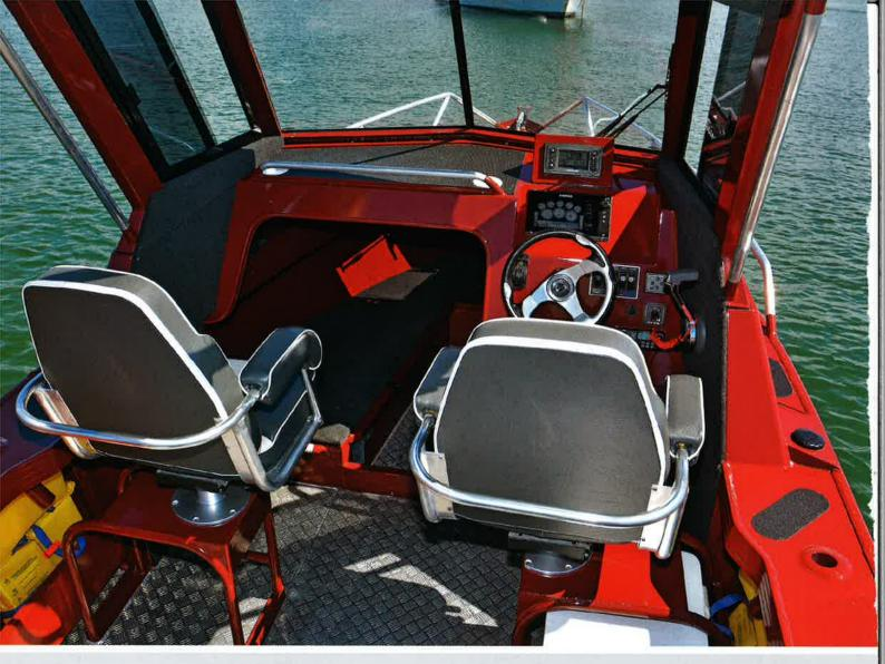
Beneath the hardtop are comfortable bucket chairs with arm rests. As standard, the chairs are mounted above aluminium frames, but they can be mounted over storage boxes. Note also the wide dash, easy cabin access, high windscreen (with wiper) and sliding side windows for ventilation.
