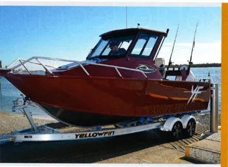
The Yellowfin 6200 boat/motor/trailer package comes in just under 2000kg and can be towed behind a regular 4WD vehicle on a trailer with standard mechanical override brakes.
