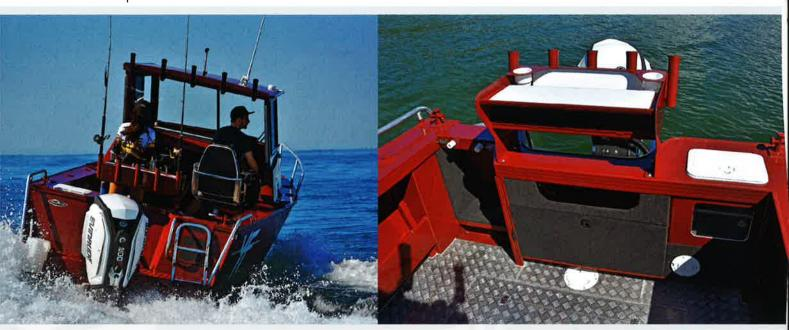
Above right: The Yellowfin 6200's self-draining cockpit is big enough for three or four anglers, and with footspace around the perimeter it offers secure footing when battling big fish. Its 60L livebait tank has a clear front viewing window so you can keep an eye on the health of your livebaits. The starboard-side transom door and the large, removable baitboard complete with rod rack are standard.
