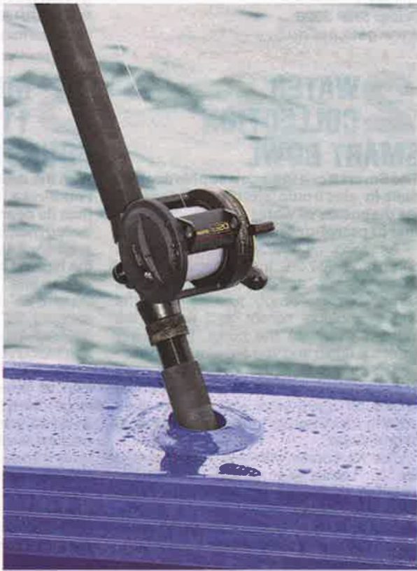
The rod holders on the gunwales are welded in including a solid gimbal at the base to give you plenty of confidence that your expensive rod and reel is going nowhere!
