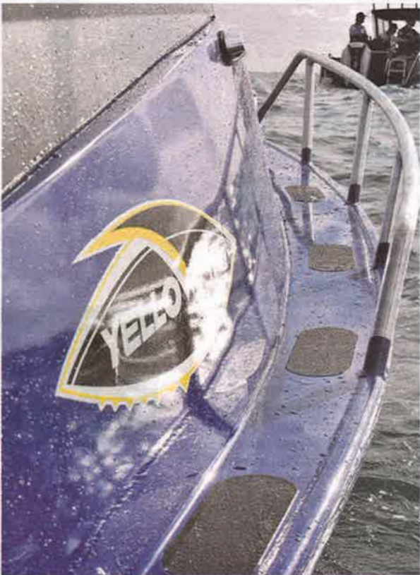
While a clumsy deckhand may stub his or her toe on the spray deflector on the side decks, they certainly do a great job of redirecting water over the side instead of into the cockpit.
