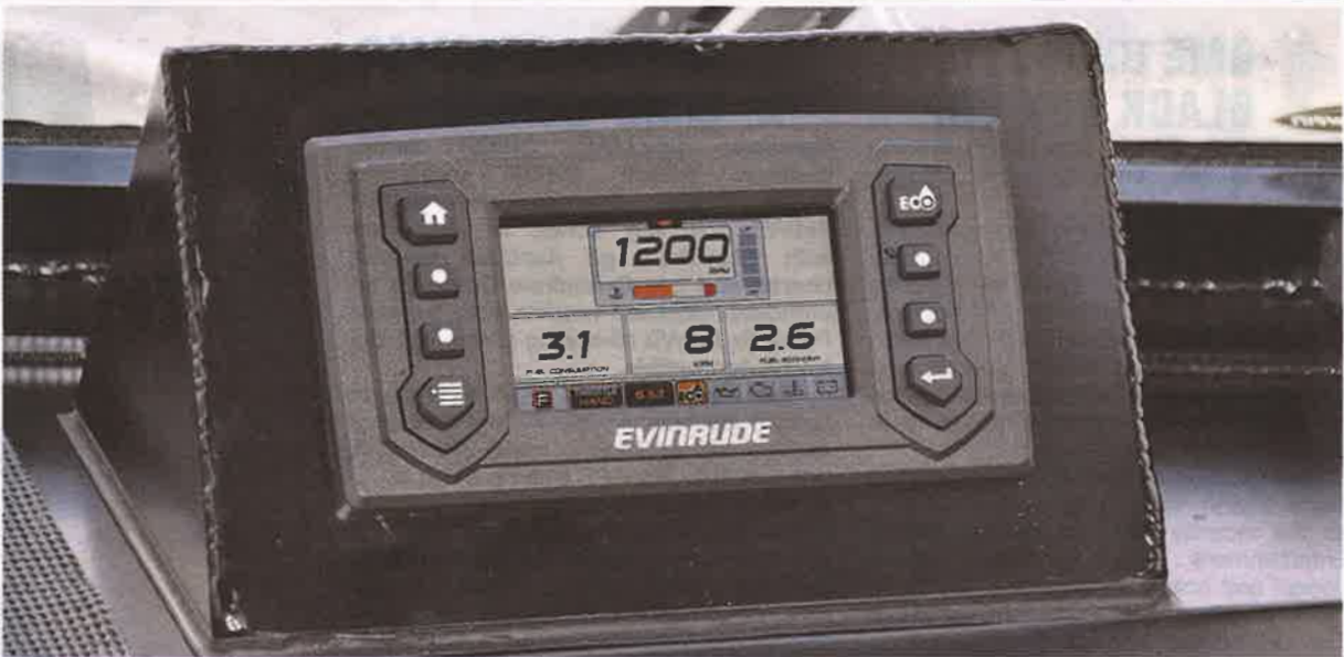
The Evinrude Icon Touch digital gauge gave super clear readings and with different page options gives the skipper the ability to quickly and easily view detailed readings of fuel/fluid levels, trip logs, engine data and more.
